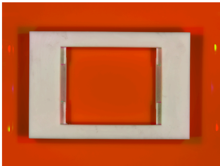
Stage, 3D-printed with white resin.
